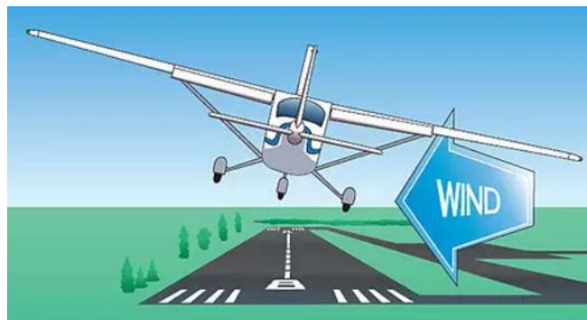
Figure 2. Aircraft attitude under the Sideslip Method.
