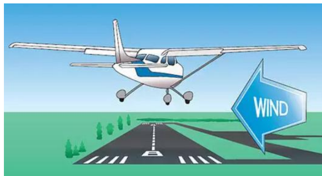
Figure 1. Aircraft attitude under the Crab Method.
