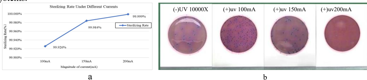
Fig. 4. Flow-Through Water Disinfection Tests at Different Currents. (a) Disinfection Rates of Flow-Through Water at Various Currents; (b) Results of Flow-Through Water Disinfection at Different Currents
