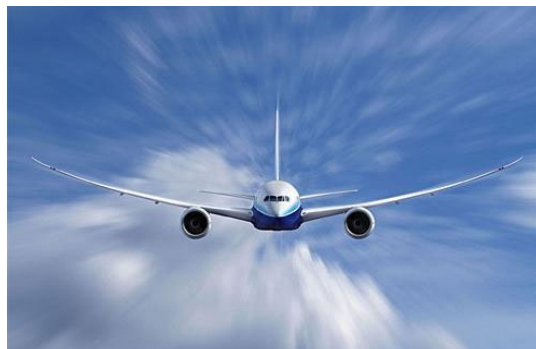
Figure 1. Static aeroelastic deformation of B787 wing.
