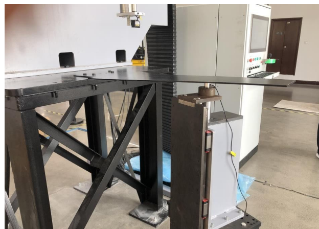
Figure 4. Flexibility Test of wing elastic model
