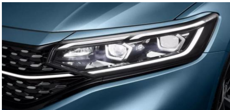
Fig 2. LED matrix headlamps
